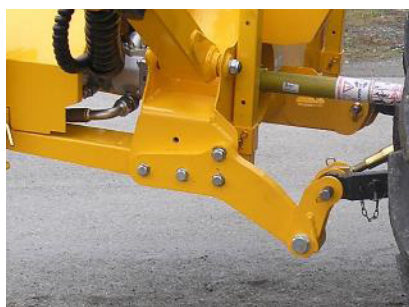
SCHOKBESTENDIGE HYDRAULISCHE BEVEILIGING MECHANICAL RELEASE SAFETY DEVICE
